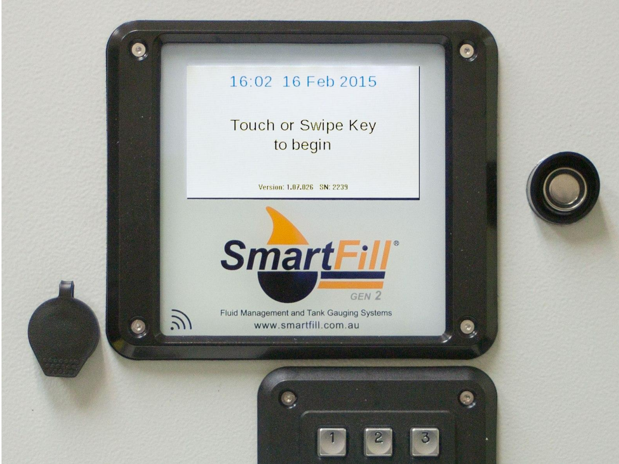
Model SmartFill GEN 2 Control System (Pattern & Variant 1) Showing Default (Idle) Screen incl. Software Version Number
